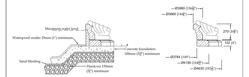
Read in conjunction with tech Sheet P11, P12 and P50 All dimensions exclude joints - allow 6mm  $(\frac{1}{4}")$  for vertical and bedding joints Unless otherwise stated, all materials other than stonework to be supplied by others
