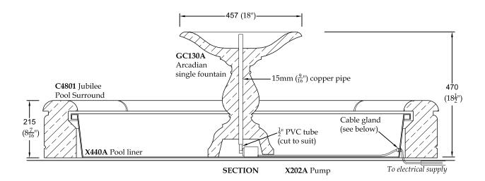
Cable Gland - Drill liner to suit. Secure gland through liner and seal with silicone sealant (not supplied).
