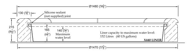
It is essential that the pool is sited on a firm and level area Foundations to suit site conditions and loadings (to be designed by others) Unless otherwise stated, all materials other than stonework to be supplied by others An 8:1 sand/cement bedding mortar should be used to avoid any pivoting or twisting strain
