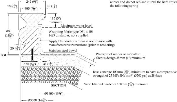
Allow 6mm  $\binom{1}{4}$  for vertical and bedding joints Unless otherwise stated, all materials other than stonework to be supplied by others
