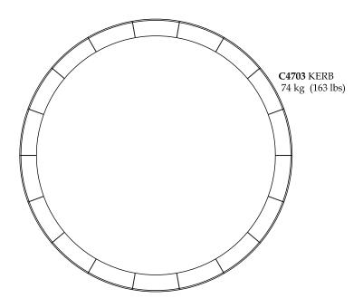
Ø 10mm  $\binom{3}{8}$ ") stainless steel dowels (not supplied) 50mm (2") projection into stone. Holes to be drilled on site to suit by others. Minimum of 2 No dowels per stone secured using a flexible building adhesive such as Evode Serious Stuff, Loctite Fast Grab, or similar
